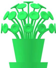
Different materials have different physical characteristics, notably fragility. Very thin parts of your design may be fragile or even unprintable. This can cause frustration, delays and damaged items.
