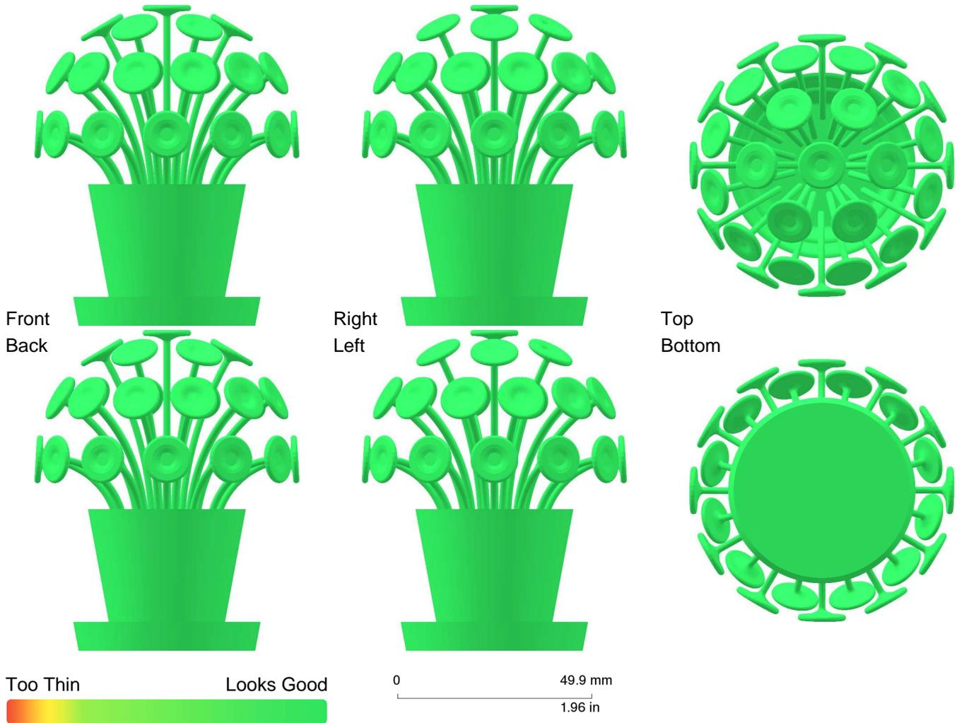
**Solidity Check** provides a heatmap of fragile areas (marked red) in your design. Despite these automatic checks, all designs go through a supplementary manual check, just to be sure.
