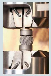
Destructive test of titanium mesh sphere in lab at ORNL [2]
